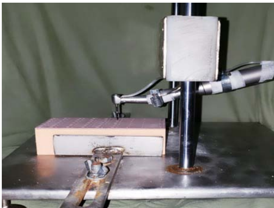
Fig. 2: Fixation of the contra-angle (20:1 reduction) on the vertical displacement device at 90° perpendicular to the specimen.
