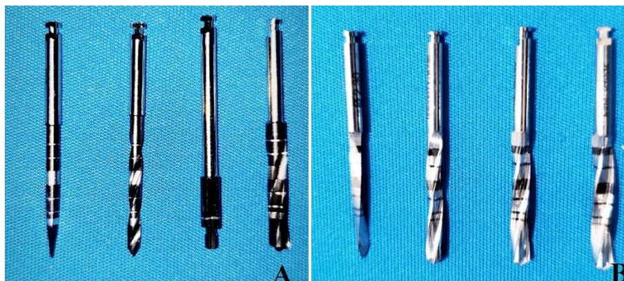
Fig. 1: (A) Drills in the Neodent group (Group N) were made of surgical stainless steel (440C). (B) Drills in the Dentoflex group (Group D) were made of surgical stainless steel (XM-16).
