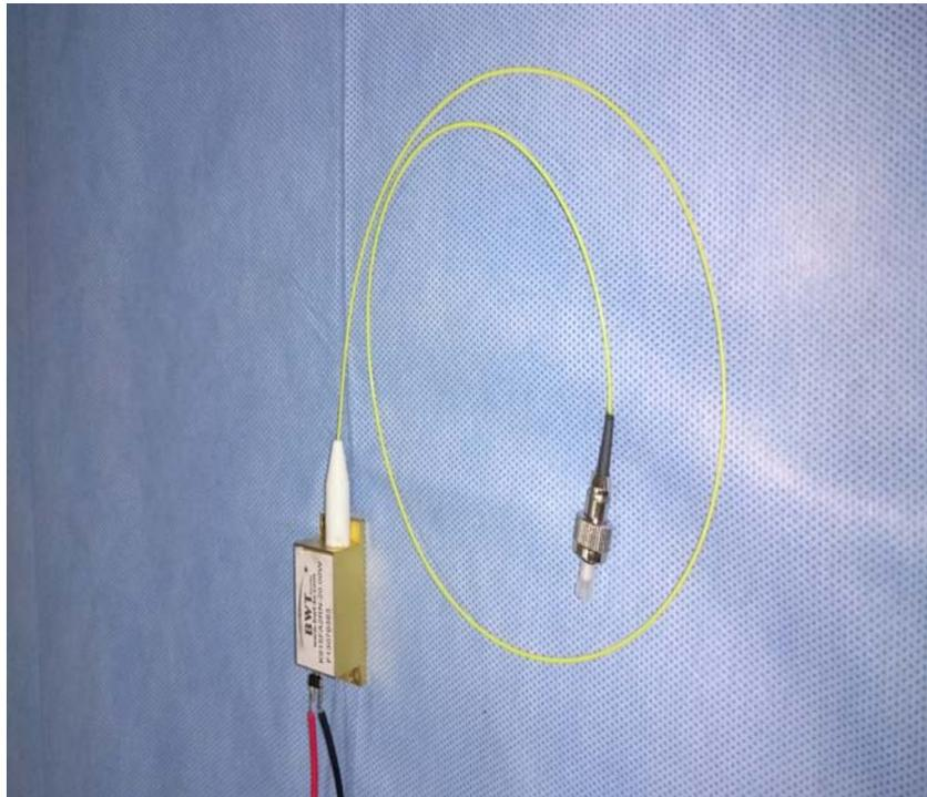
Photo 3: Laser diode coupled with 0.1 mm optical fiber
