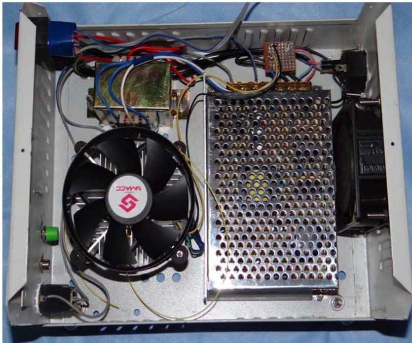
Photo 4: Showing inner view of the machine-Laser diode with cooling fan and power supply
