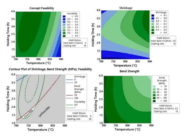
*Figure 7:* Contour diagrams of Flexural strength, feasibility, shrinkage and the overlap diagram with combination of high values
