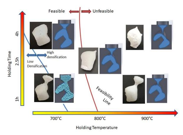
*Figure 5:* Comparison diagram of concept feasibility as a function of Holding temperature and holding time
