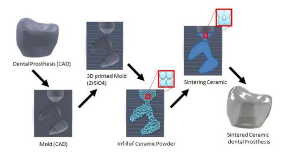
*Figure 1:* Schematic of ceramic dental prostheses based on ZrSiO4 – Glass composites fabricated by indirect Additive manufacturing
