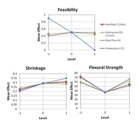
Figure 4: Standardized Main effect of control factors on Feasibility, Flexural strength and shrinkage
