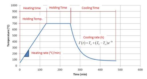
Figure 2: Illustration of sintering temperature curves and control factors: Holding Temperature (T<sub>hold</sub>), holding time (t<sub>hold</sub>), cooling rate (k) and heating rate (Hr)
