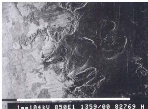
Figure 7 : Scanning electron micrograph of a fluoride-modified implant after the push-out procedure. The implant is partly (right side) covered by bone that is firmly fixed to the implant surface, which indicates bonding between the titanium implant and bone
