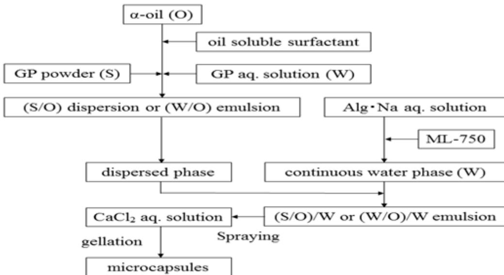
Figure 1 : Flow chart for preparing microcapsules
