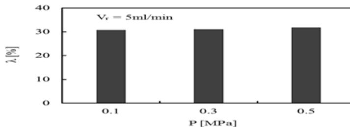
Figure 8 : Dependences of Microencapsulation Efficiency of Spraying Pressure
