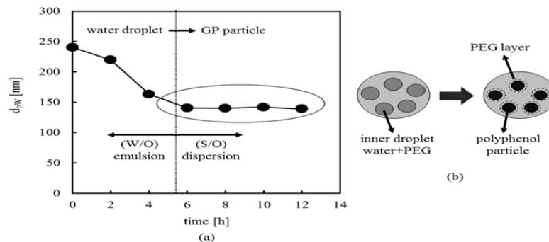
Figure 11 : Transient Inner water Droplet Diameters
