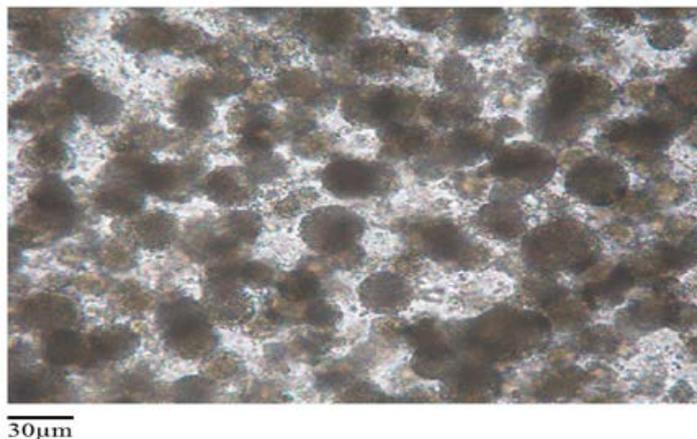
Figure 5 : Optical Microscopic Photographs of (W/O)/W Emulsion
