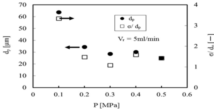
Figure 7 : Dependences of mean Diameter and Dispersion Degerr on Spraying Pressure
