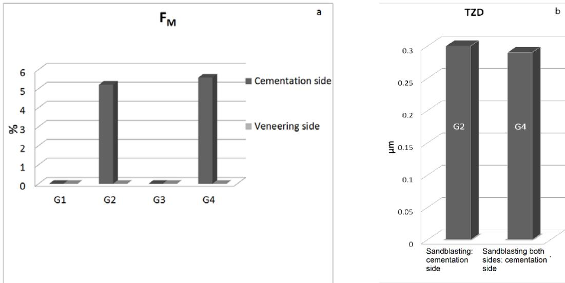
Figure 1: (a) Relative amount of monoclinic phase ( $F_M$ ) revealed by XRD on zirconia surface after different surface treatment. (b) Transformed zone depth (TZD) on zirconia sandblasted without porcelain sintering cycle.
